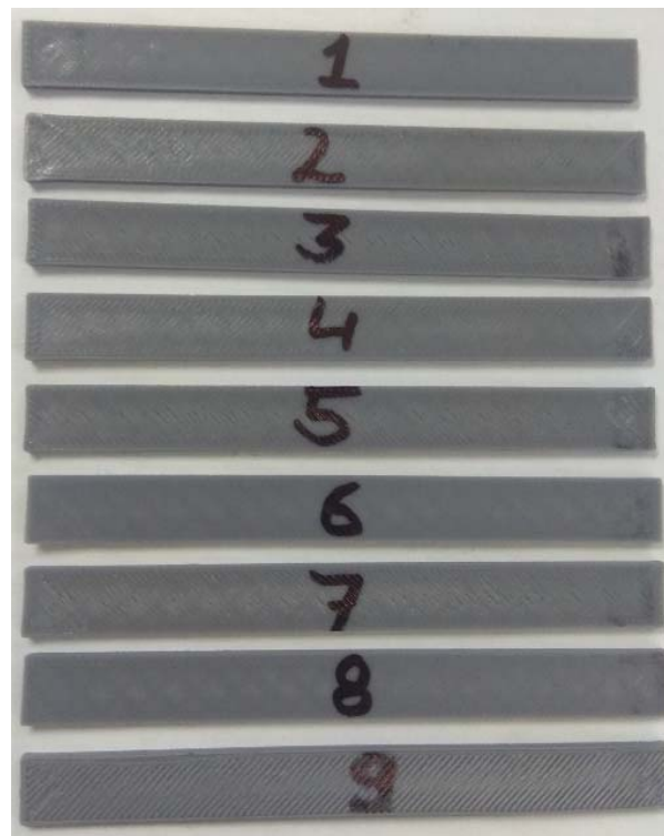
Figure 3. Rectangular shaped PLA samples
